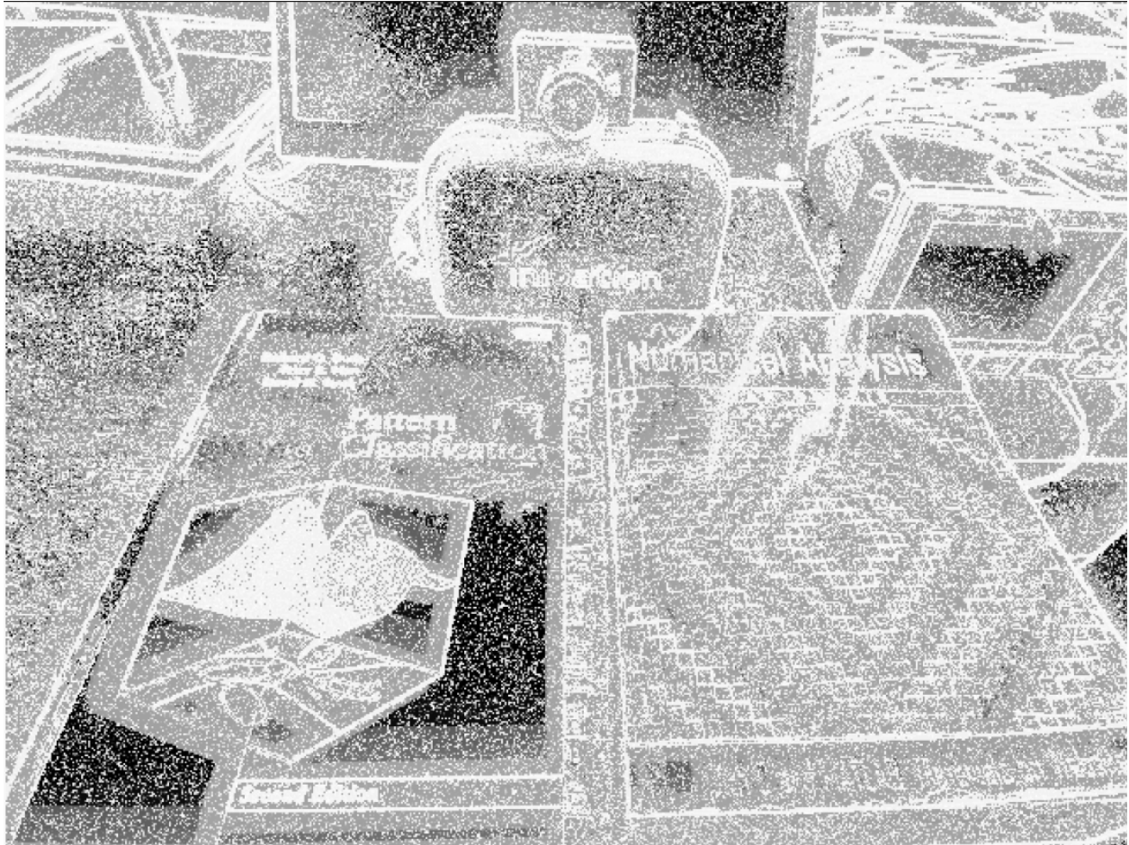
Fig. 6: Frame generated using dv::TimeSurface class.
