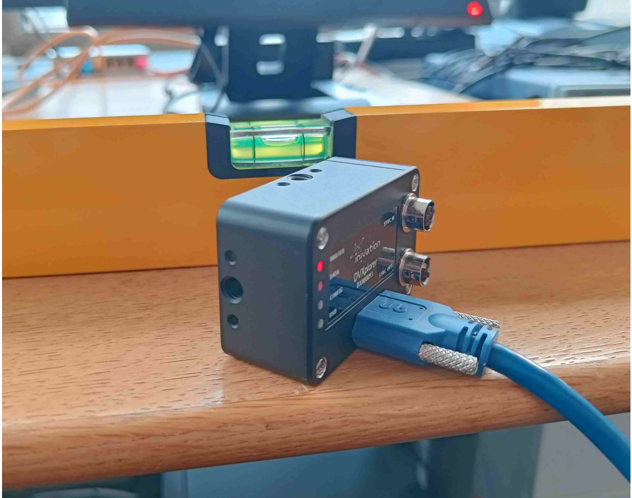
Fig. 15: Camera placed on a level table surface for imu bias estimation.
