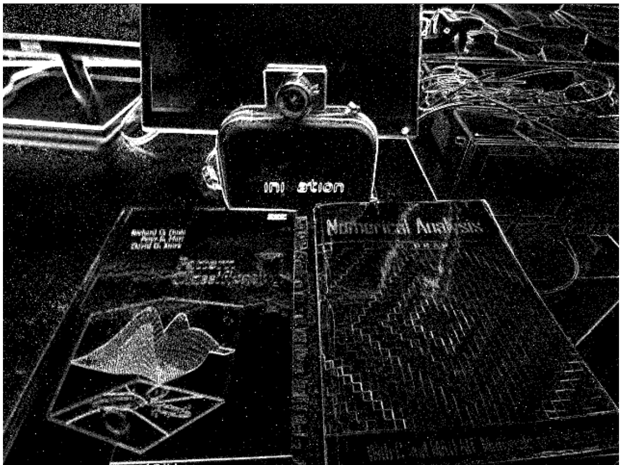
Fig. 1: Frame generated using dv::EdgeMapAccumulator class.
