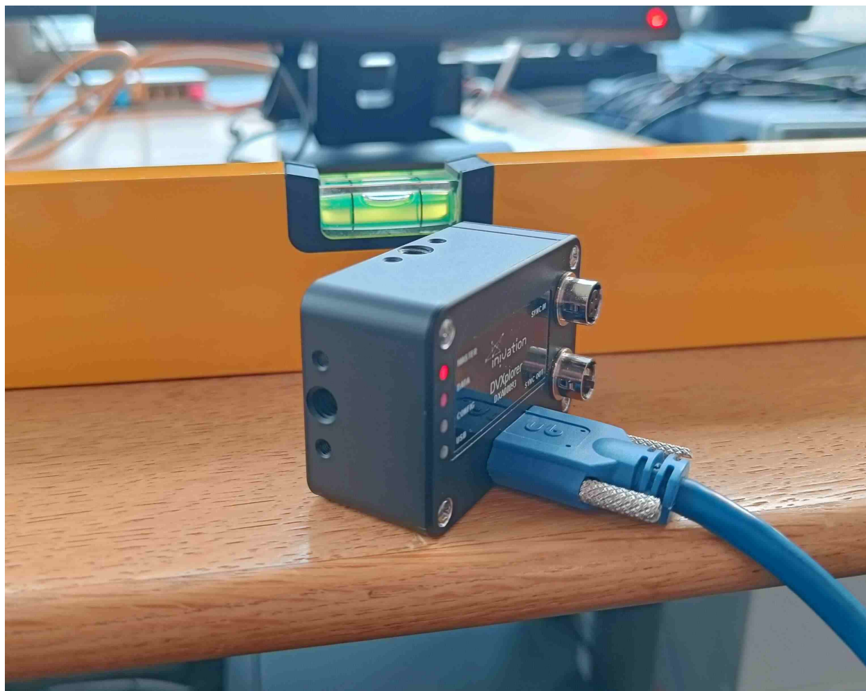
Fig. 15: Camera placed on a level table surface for imu bias estimation.
