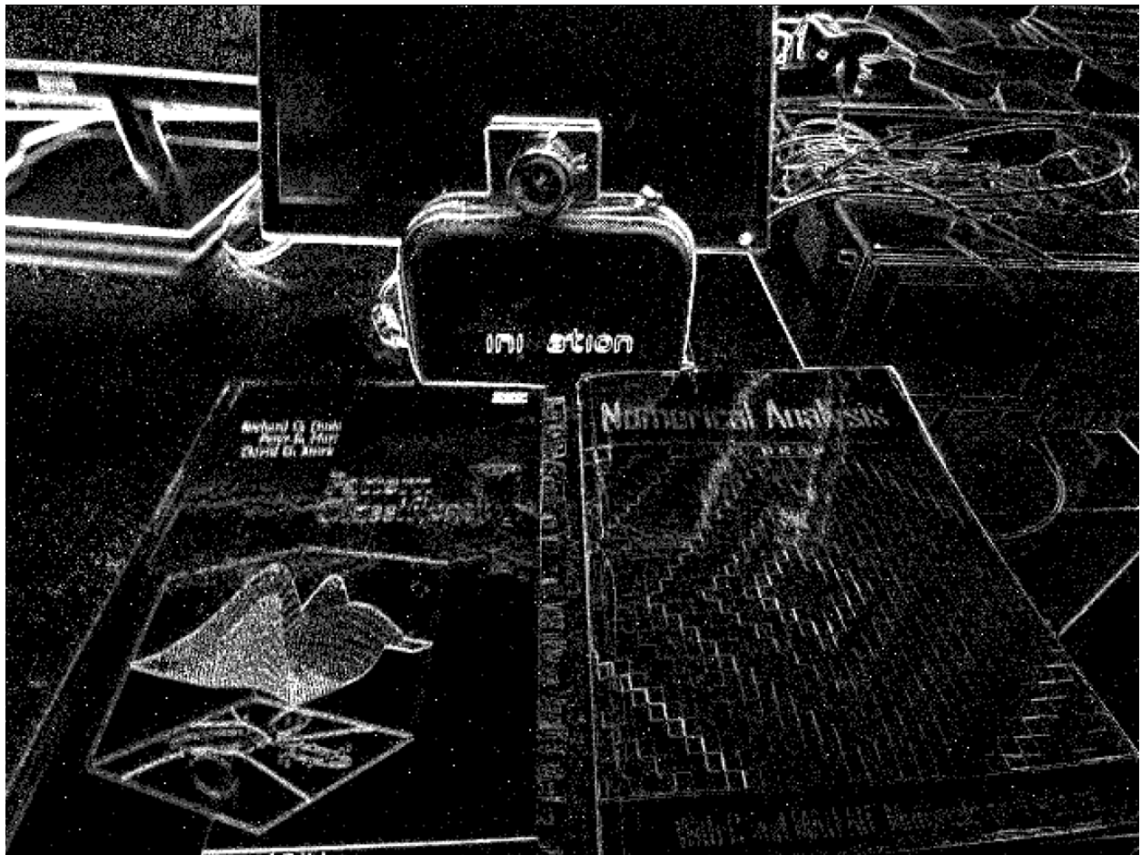
Fig. 1: Frame generated using dv::EdgeMapAccumulator class.
