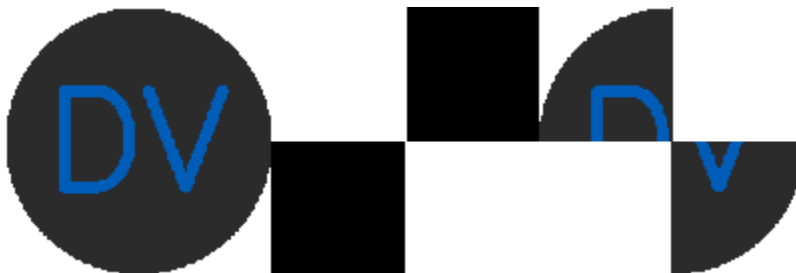
Fig. 11: Output of the sample use of event mask filter. Left is a preview of input events, middle is the mask used, and right is a preview of filtered events.
